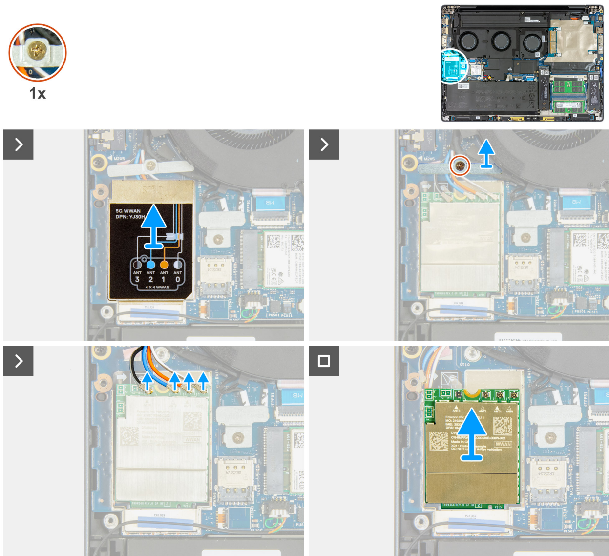
Figure 48. Removing the WWAN card
