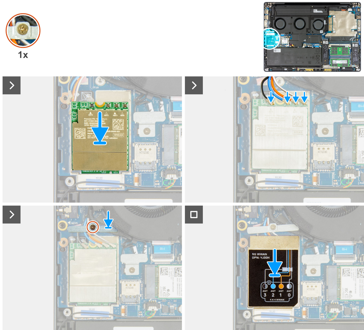
Figure 49. Installing the WWAN card
