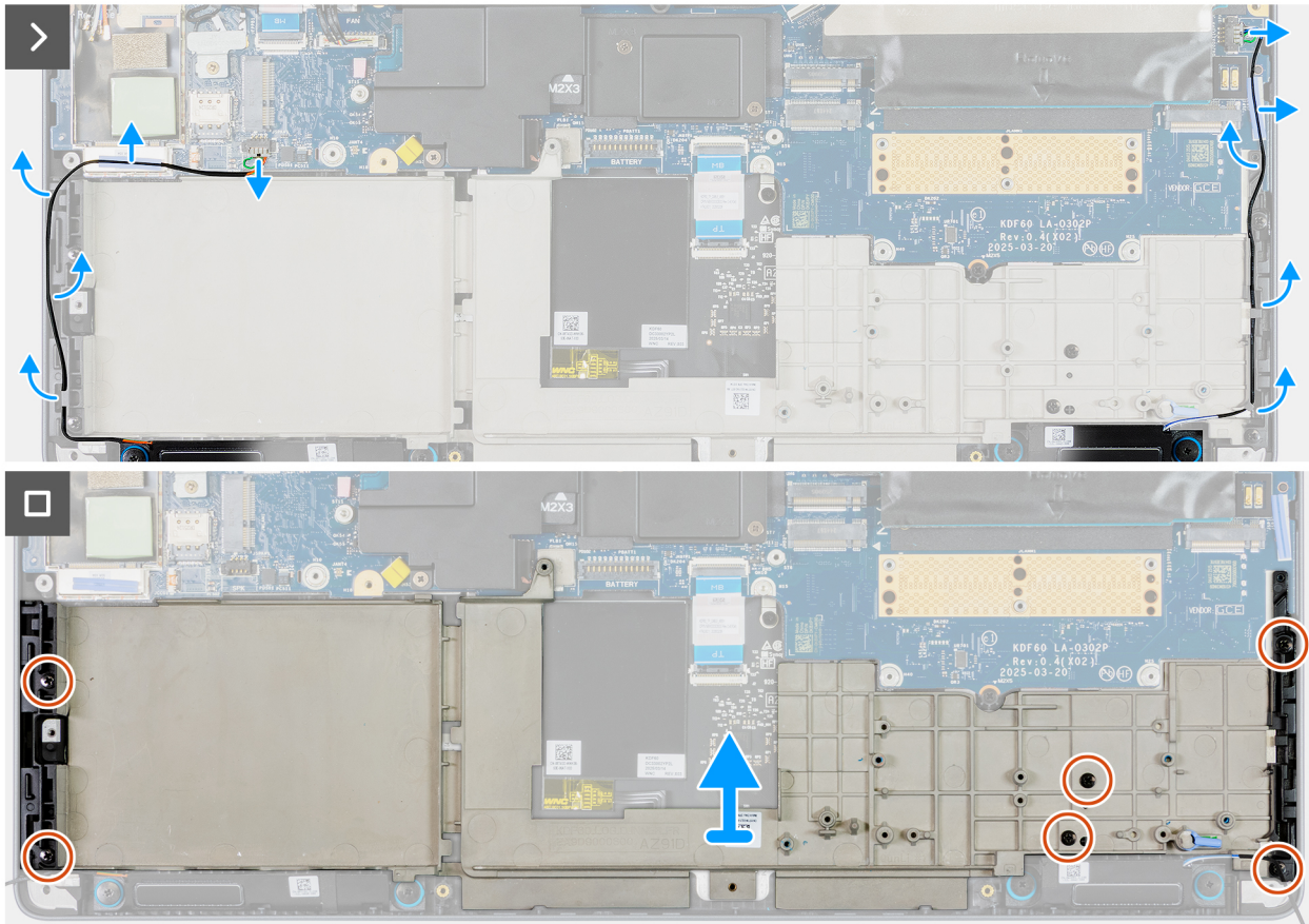
Figure 82. Removing the inner frame
