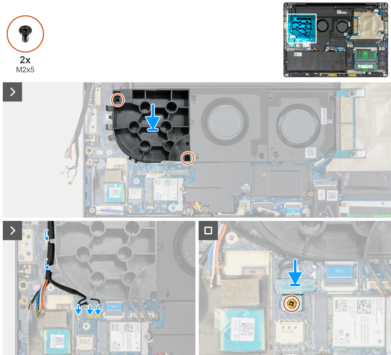
Figure 58. Installing the dummy fan
