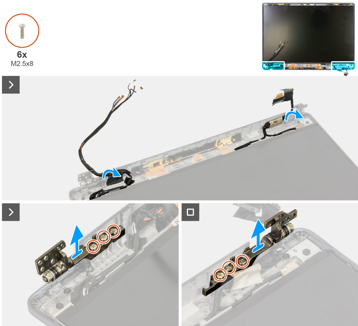
Figure 102. Removing the display hinges
