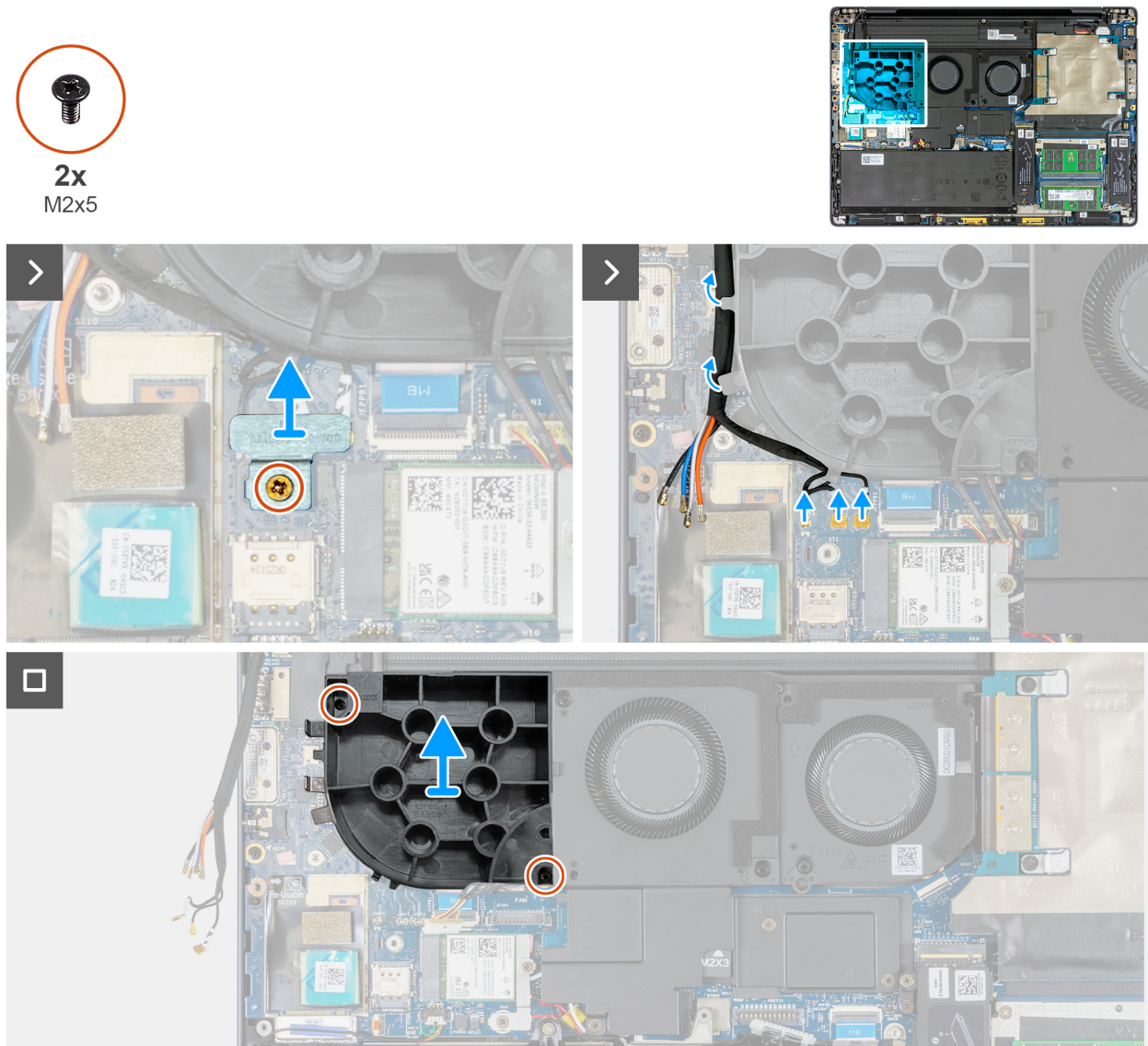
Figure 57. Removing the dummy fan
