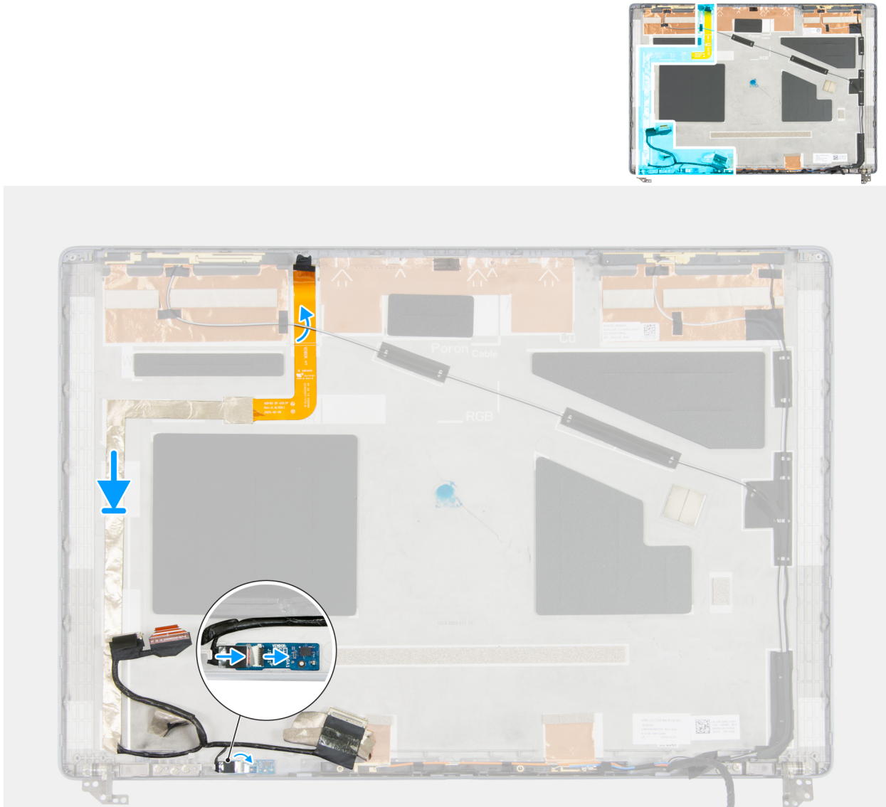
Figure 108. Installing the display cable
