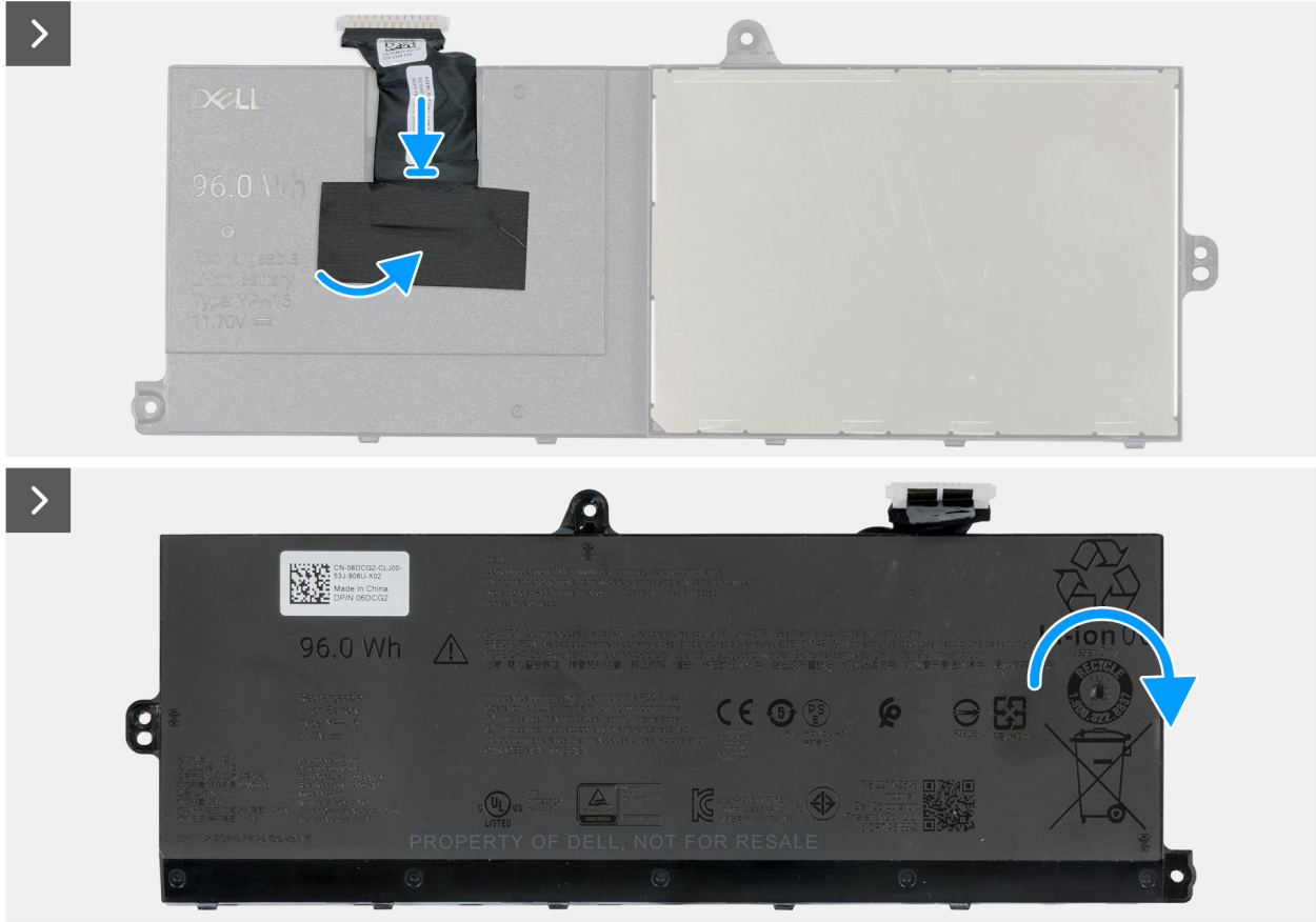
Figure 40. Replacing the battery cable
